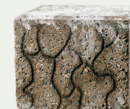
Efflorescence emerged from pores within a magnified area of a concrete paver. The calcium has been carried to the surface by water.
